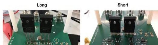
Figure 4. Long lead (left) vs. short lead (right). Short lead is recommended whenever possible.
