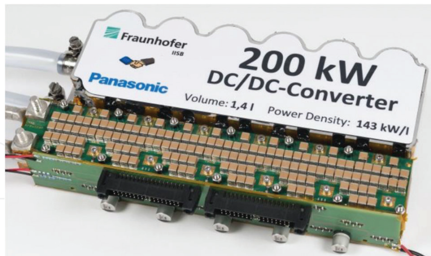
Figure 19. A 200kW full-SiC converter presented by Fraunhofer. The converter achieves an impressive power density >100\text{W}/\text{cm}^3 switching at 200kHz, with an efficiency of 98.9%.
