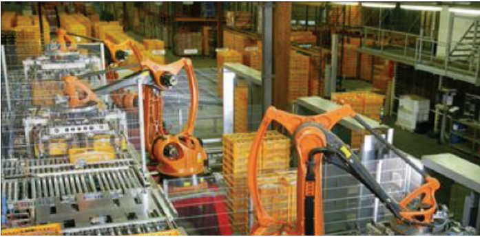
Figure 1: Industrial robots are used for palletizing food products like bread and toast at a bakery in Germany. (Source: Mouser)
