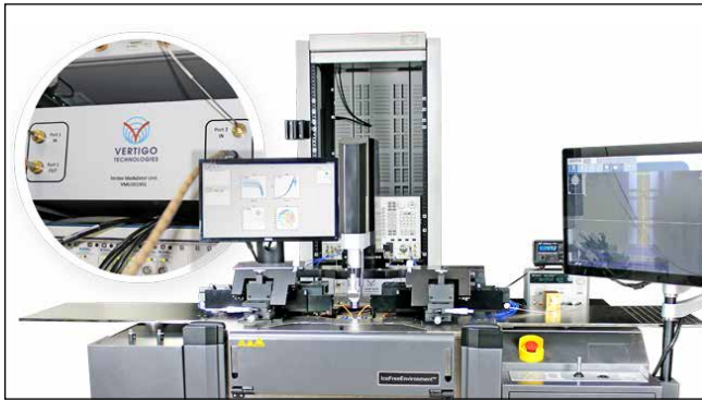
▲ Fig. 10 Active load pull up to 1.1 THz with their strategic partner Vertigo Technologies and our MMW-STUDIO solution.
