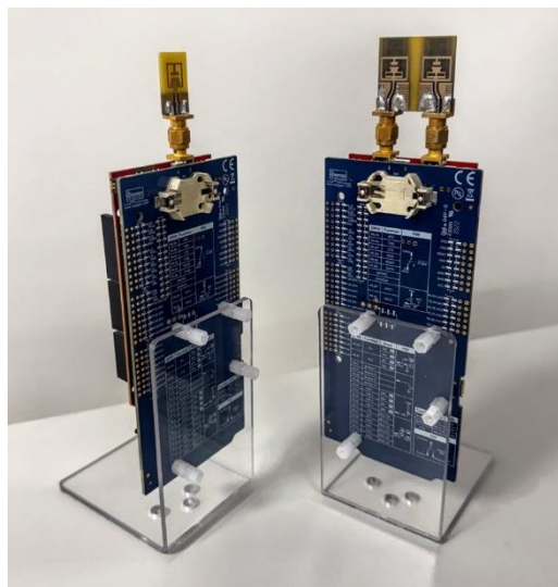
Figure 4. QM33110 board with omni-directional antenna and QM33120 board with AoA antenna
