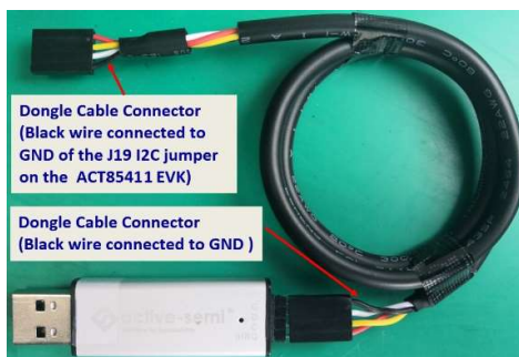
Figure 4 USB-TO-I2C Dongle Connection
