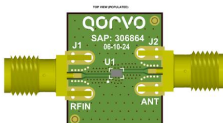
Figure 2a. QPQ5501 Evaluation Board PCB
