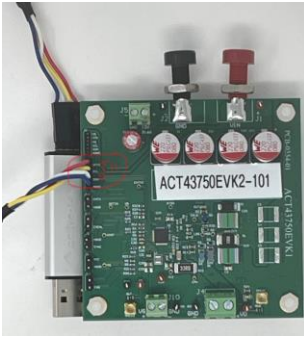
Figure 3. Old dongle connection at J11
