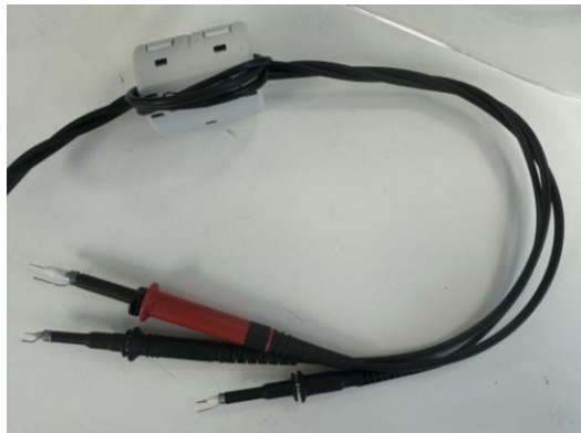
Figure 23 Filtering common mode gate to source noise with ferrite core on twisted wires
