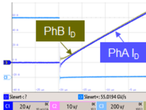
Figure 2 Dynamic current mismatch due to threshold voltage mismatch
