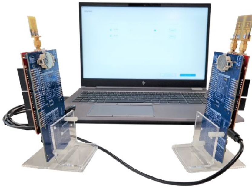
Fig. 1.7: QM33120WDK1 evaluation set-up
