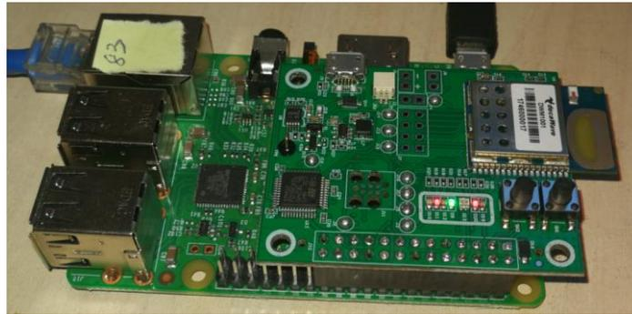
**Figure 15: Connecting DWM1001 to Raspberry Pi 3 over header pins**
