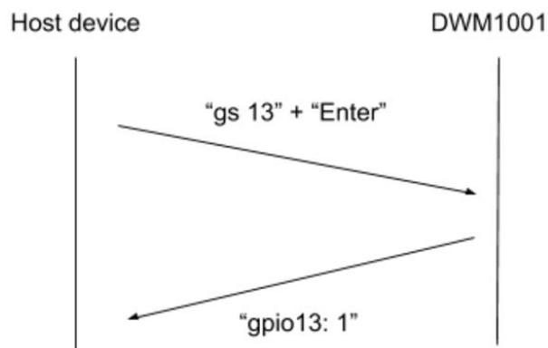
Figure 10 UART example: Shell mode communication
