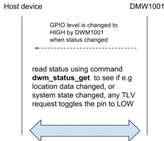
**Figure 11 GPIO scheme: DWM1001 notifies host device of status change, using GPIO**
