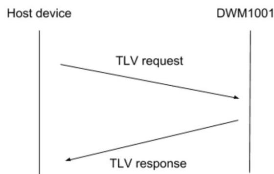
Figure 7 UART scheme: TLV mode communication
