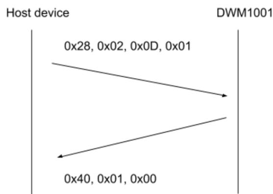
Figure 8 UART example: TLV mode communication
