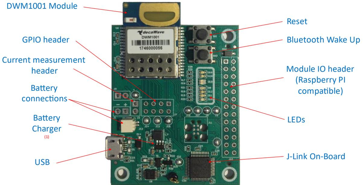
(1) Battery Charger not mounted on boards shipped after November 2021
