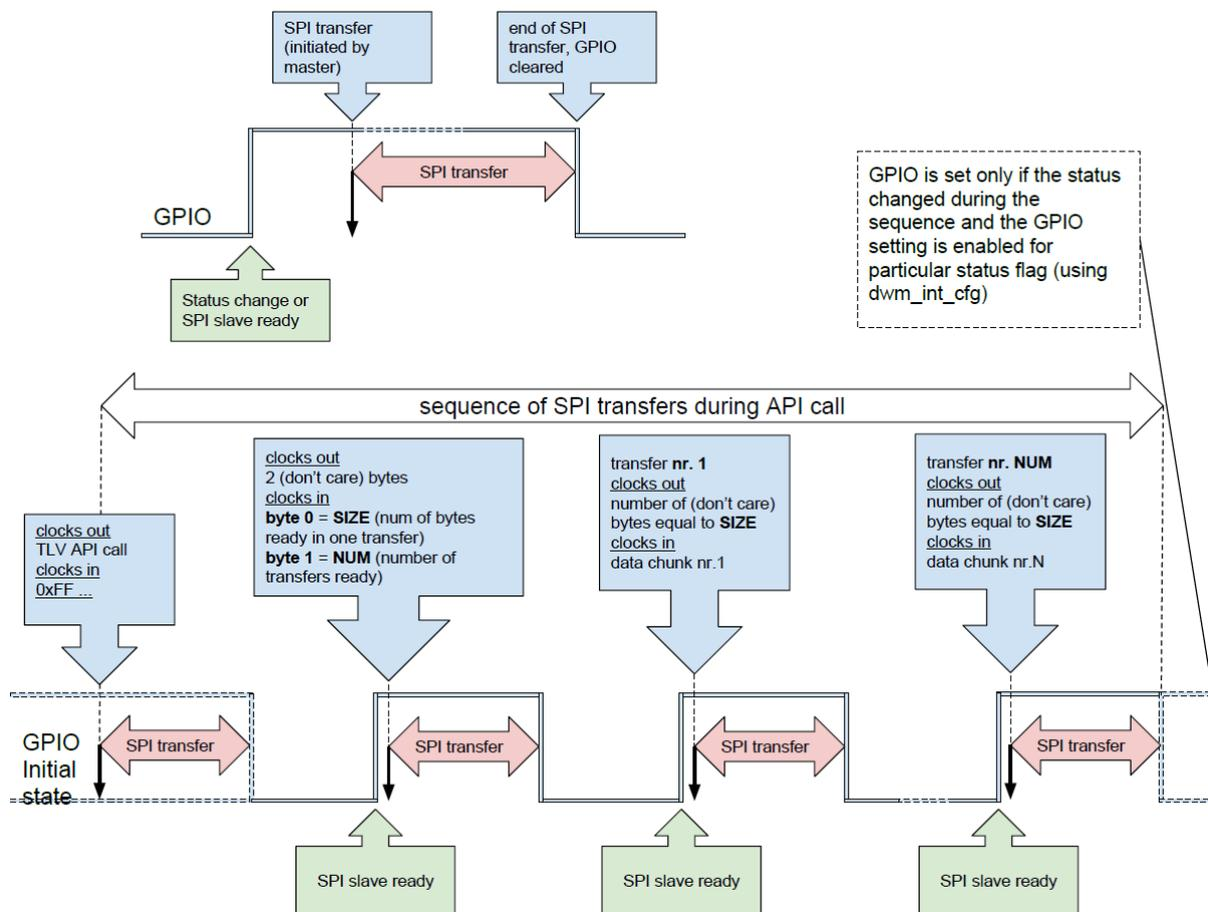
Figure 5 SPI scheme: TLV communication using data ready pin
