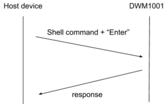
Figure 9 UART scheme: Shell mode communication
