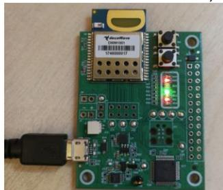
**Figure 6 DWM1001 DEV board – micro USB connection**
