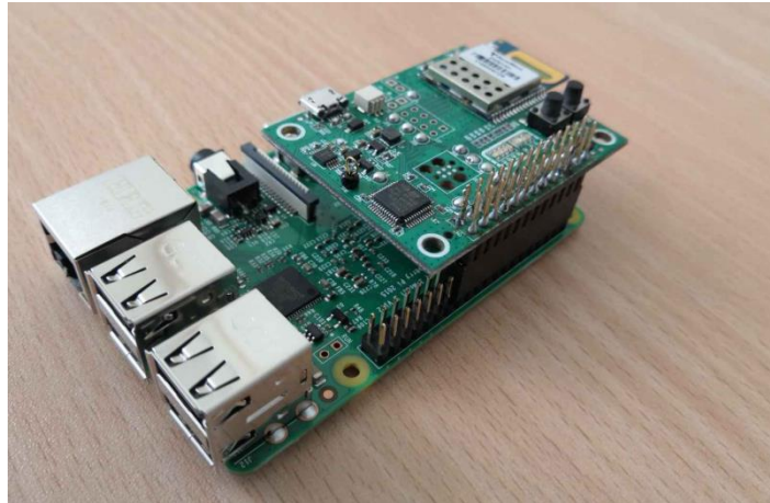
Figure 10: Gateway: R3B plus bridge node (DWM1001-DEV)
