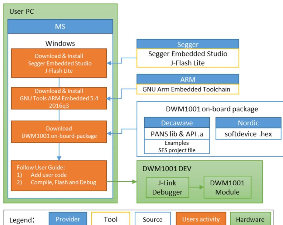
**Figure 3: Tool chain and source components in DWM1001 firmware development**
