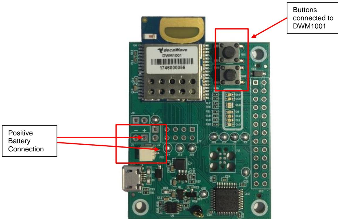
Figure 12: Picture of the module development board showing the battery connection points and buttons
