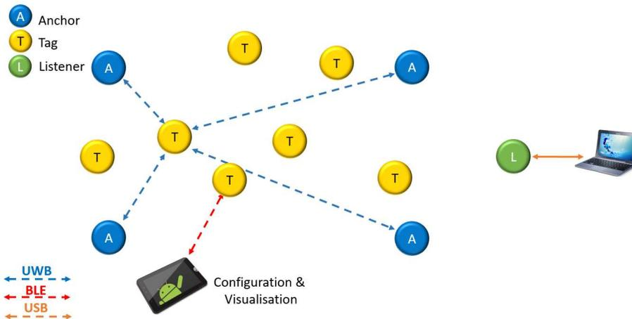
A PC can be used to connect directly via USB to a tag or to an RTLS unit configured as a listener in order to collect and log the location data from the tags. This can be done using a terminal interface.
