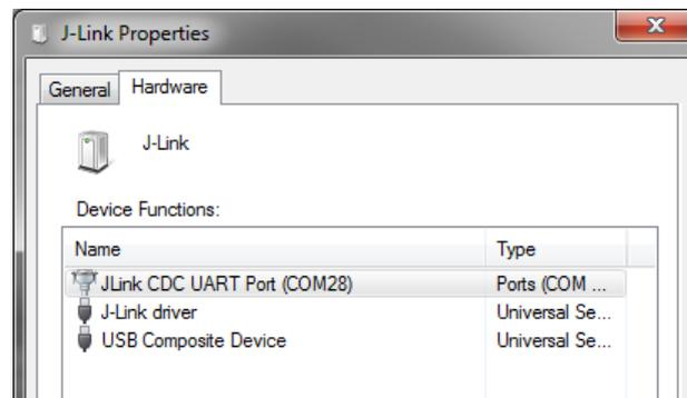
**Figure 14: DWM1001 Device COM port over J-Link**
