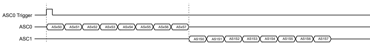
Figure 17-5. ASCx, ADCCTL.ADCMODE = 011b, 110b
