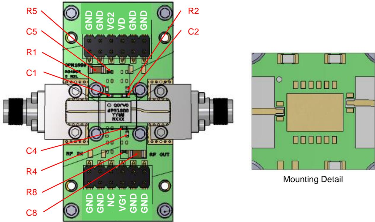
RF Layer is 0.008" thick Rogers Corp. RO40003C ( $\epsilon_r = 3.35$ ). Metal layers are 1.0 oz. copper. The microstrip line at the connector interface is optimized for the Southwest Microwave end launch connector 1092-01A-5.
