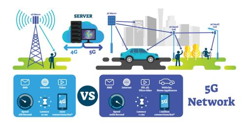
5G network performance improvements are due to new mmWave antenna configurations with active beam steering
