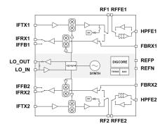
The half-duplex Transceiver ICs integrate dual Tx single-sideband up-conversion, dual Rx image-reject down-conversion functionality, and an on-chip synthesizer that enables 2T2R applications within a single die.
