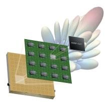
Anokiwave, now Qorvo, invented the quad BFIC architecture, which allowed symmetric implementation of phased array antennas with high volume/ low-cost scalability, that are used in mmWave systems enabling a much lower cost point. Over its history, Anokiwave, now Qorvo, has delivered millions of ICs with more than 95% cost reduction. The ICs meet various AESA antenna requirements with proven performance in commercially deployed SATCOM terminals and 5G systems.
