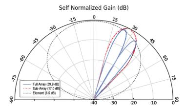
Figure 14: Hybrid Beamforming Beam Illustration
