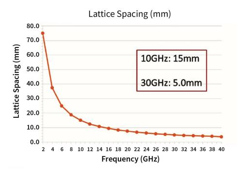
Figure 9: Lattice Spacing Example Calculation
