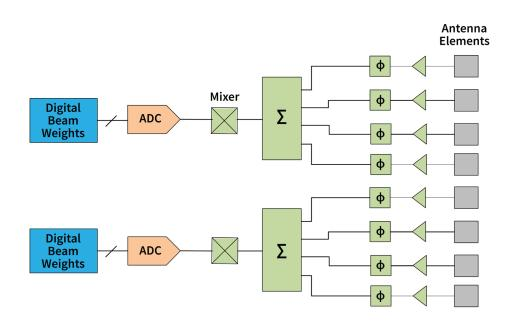
Figure 13: Receive Hybrid Beamforming Block Diagram
