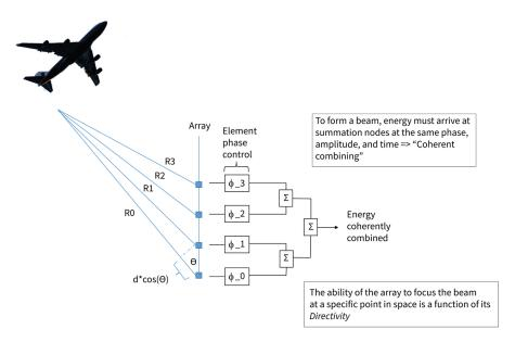
Figure 2: Coherent Summation of Energy - Linear Array
