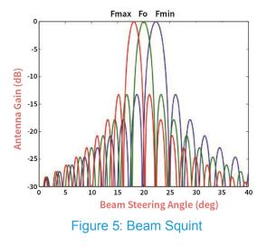
Another characteristic of all active antennas is the loss of aperture gain as the beam is steered away from the boresight direction — defined as  $\Theta$ =0. This characteristic, called scan loss, follows 10\*log(cos<sup>N</sup>( $\Theta$ )) power, where  $\Theta$  is the scan angle off boresight and N is a numeric value, typically in the 1.3 range, which accounts for the non-ideal isotropic behavior of the embedded element gain.
