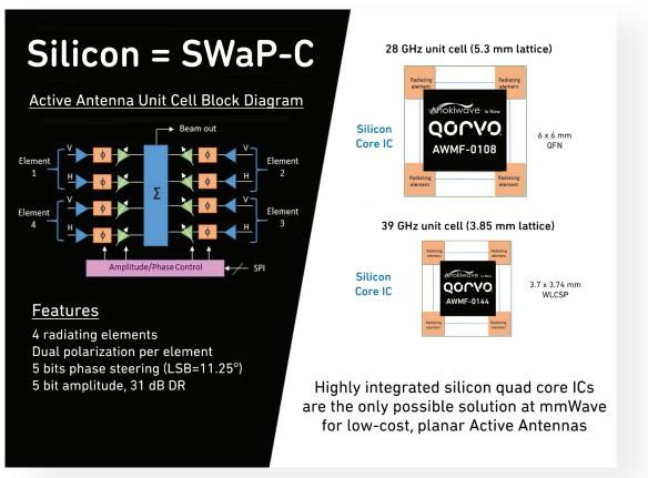
Figure 10: Highly integrated silicon ICs are critical to achieve planar active antennas at mmWave frequencies
