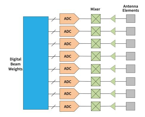
Figure 12: Digital Beamforming Block Diagram
