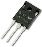
UnitedSiC cascode FETs utilize a low voltage MOSFET to turn the Normally-On JFET to a Normally-Off device with the Gate drive behavior of a Silicon MOSFET.
