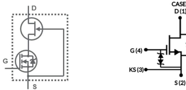
**Figure 1:** (left) Basic Cascode diagram showing the MOSFET drain connected to the JFET source. (right) Cascode diagram showing back-to-back diodes on the Gate to Source pads of the MOSFET.
