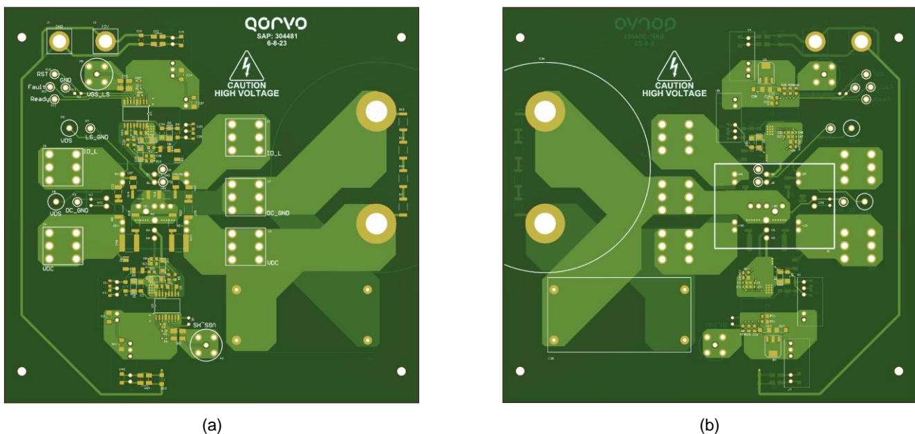
Figure 4. Half-bridge E1B module DPT EVB 3D view. (a) top view and (b) bottom view.
